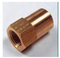
The B-25 Nozzles are of two piece construction with large tangential metering slots in the internal Disc to give a nonrestrictedflow with a uniform "Solid" distribution. Sizes from 3/8" NPT to 3/4" NPT are made from bar stock while larger sizes are castings. For special applications, a hollow cone spray can be produced from this same design. These Nozzles with high flow rates and coarser sprays are used in gas scrubbing, adsorption towers, brine spraying, and chemical and industrial processing.
